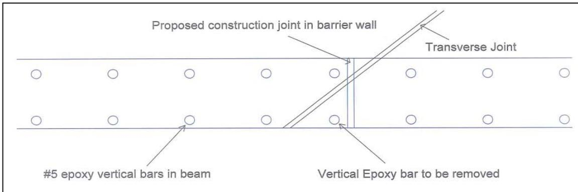
Figure 12 - Rebar Cut on Skewed Beam
