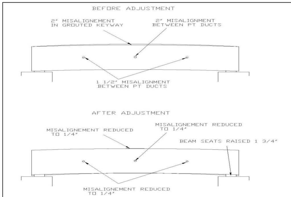
Figure 6 - Adjusting Beams to Align Post Tensioning Ducts
