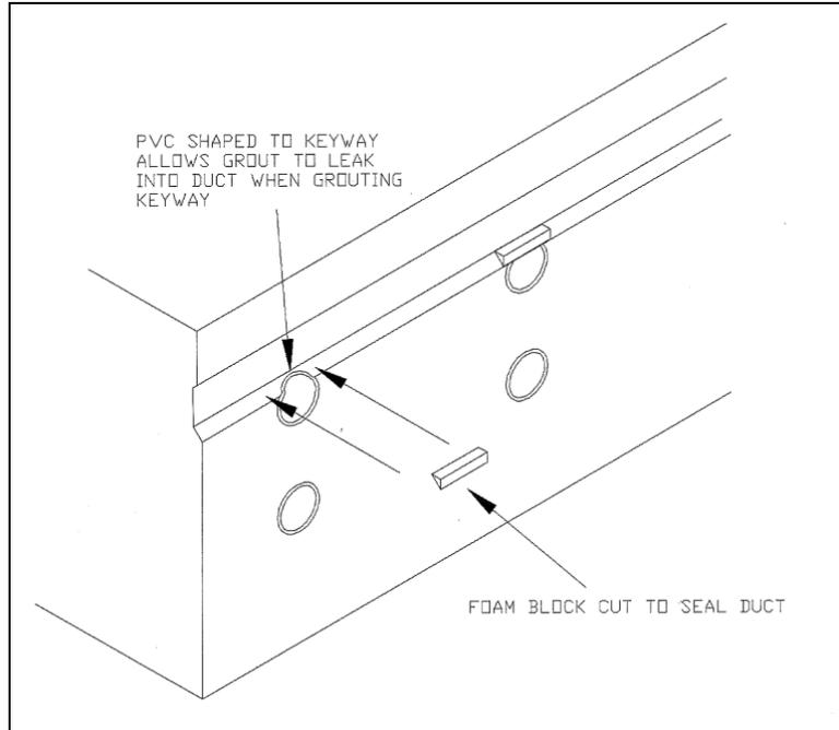
**Figure 2 - Half Keyway Glued Above Conflicting Duct**
