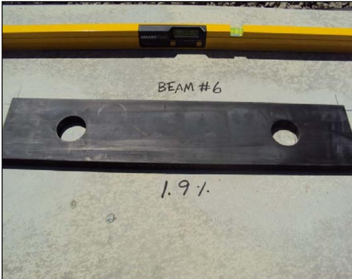
Figure 4 - Documenting Slope of Beam Seat with Smart Level
