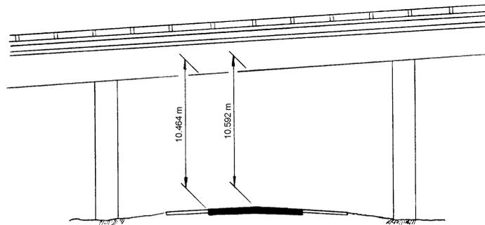
Highway 10.464 meters beneath structure
