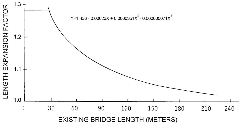
**REPLACEMENT BRIDGE LENGTH = EXISTING BRIDGE LENGTH x LENGTH EXPANSION FACTOR**
