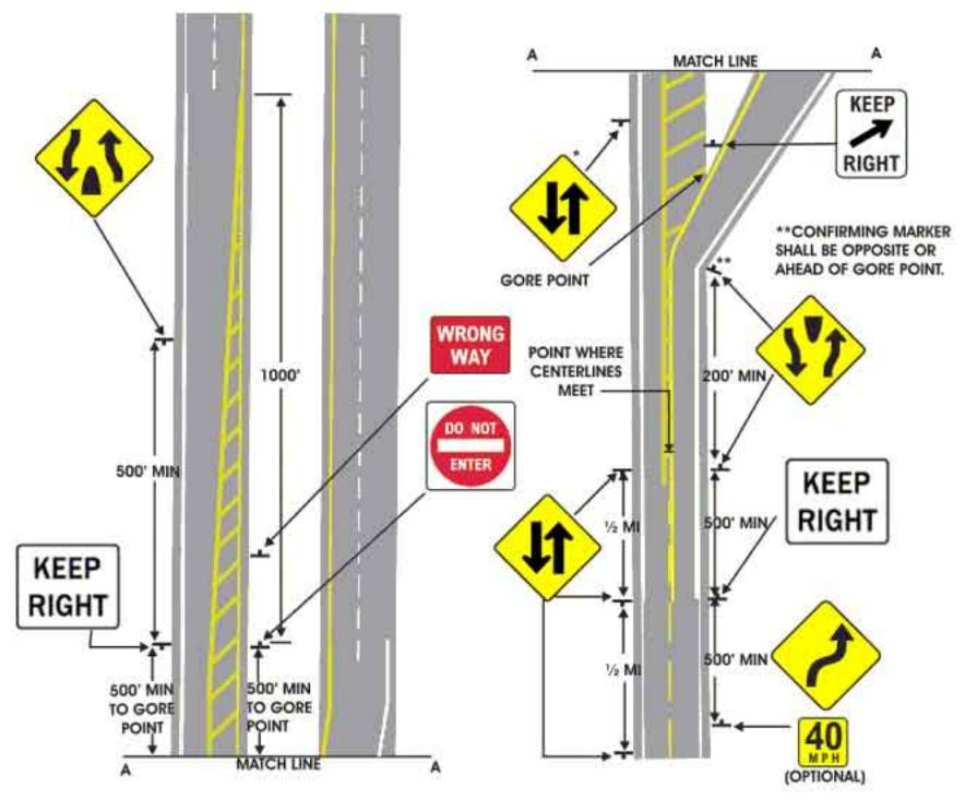
\*TWO ADDITIONAL "TWO WAY TRAFFIC" SIGNS SHALL BE PLACED AT 3 MILES AND 5 MILES FROM THE POINT WHERE THE TWO CENTERLINES MEET (OR END OF DIVIDED HIGHWAY) WHEN THE FOLLOWING CONDITIONS EXIST.
