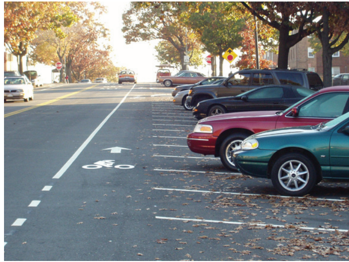
Figure 4-15. Example of Bike Lane Adjacent to Back-in Diagonal Parking (Photo courtesy of William Schultheiss of Toole Design Group.)
