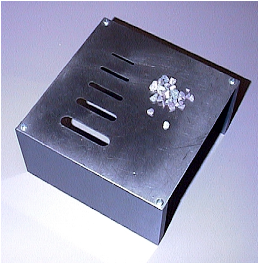
Figure 4.6. Flakiness Index Testing Plate
