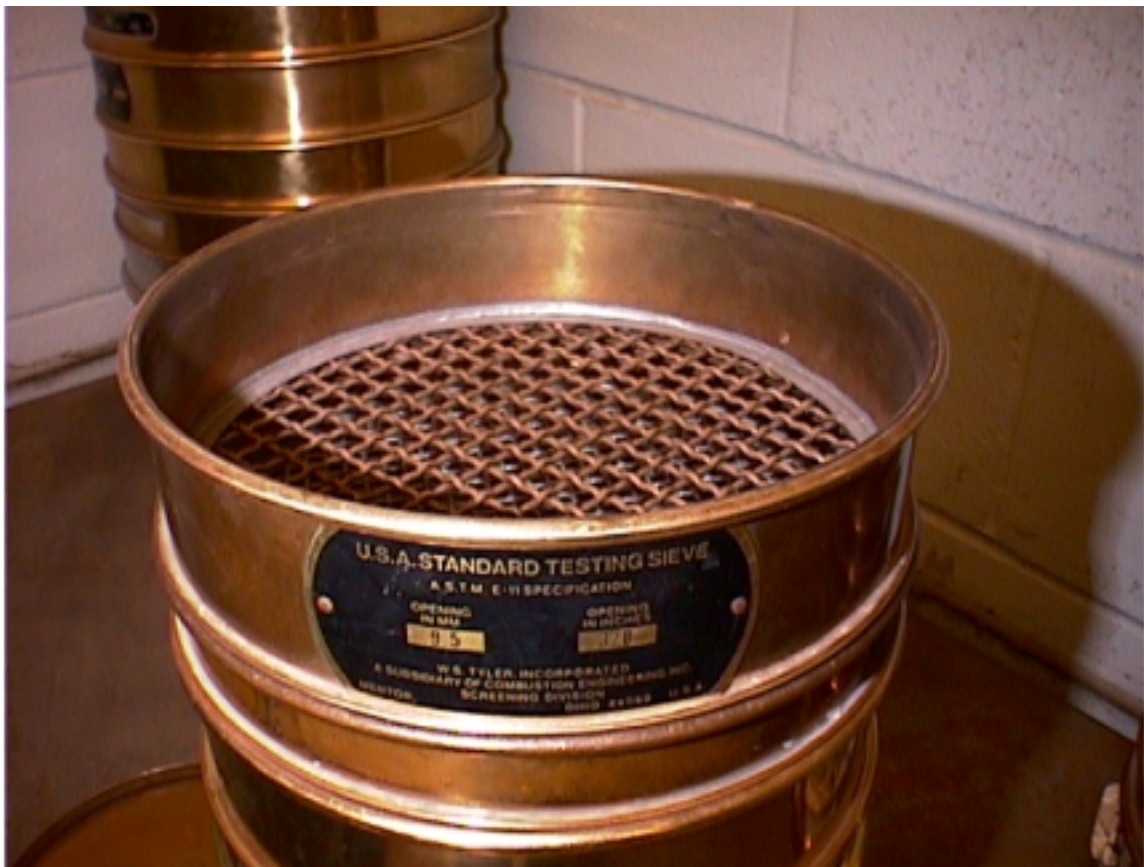
Figure 4.5. Seal Coat Sieve Nest
