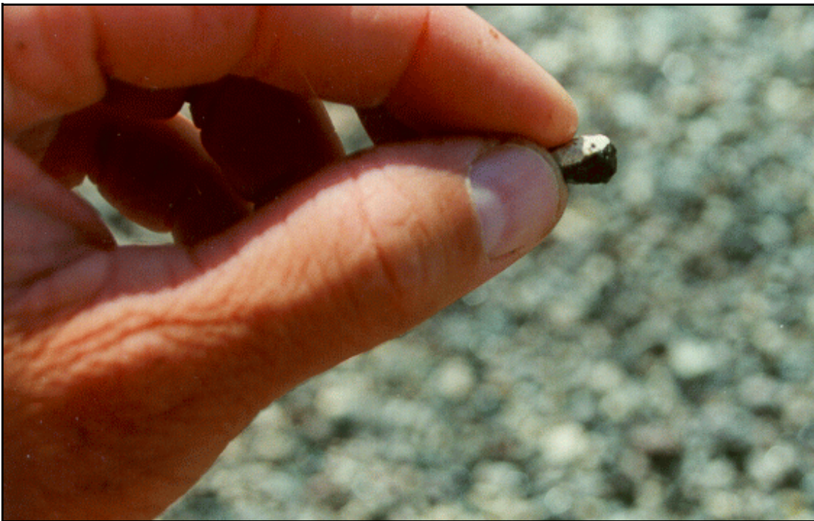
Figure 4.4. Proper embedment (~70%) into the residual asphalt.
